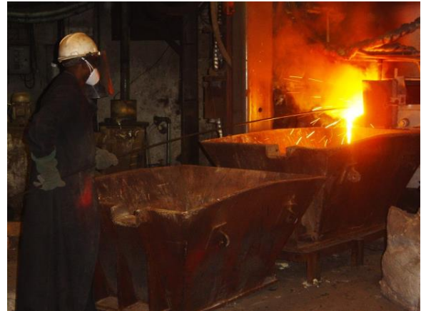
(b) A furnace operator lancing a furnace taphole on a 200 kVA DC furnace at Mintek. (Photograph: IJ Geldenhuys, Mintek, 2004)
