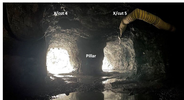
Figure 4—Photograph showing a pillar left between two cross-cuts at an intersection in a large span (Vermeulen, 2024)
